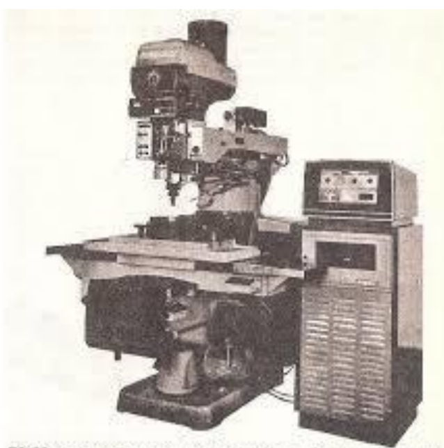
FIGURE 7.2 NC system showing machine tool and controller. (Courtesy of Bridgeport Machines Division of Tiedman Inc.)
