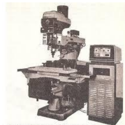
FIGURE 7.2 NC system showing machine tool and controller. (Courtesy of Bridgeport Machines Division of Textron Inc.)
